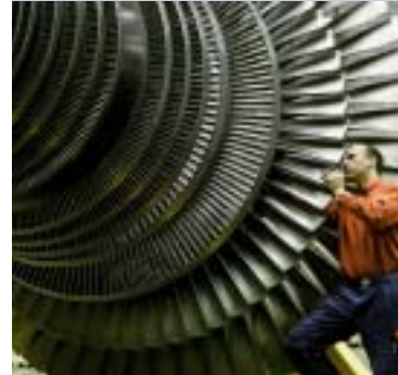
Barranco, Gran Canaria, 82 MW SST-900 for combined cycle power generation
